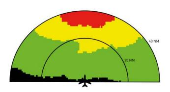
Class A TAWS system as defined in DO-367 and TSO-151D provides aural warnings and cautions for Ground Proximity Warning - GPWS functionality including;
